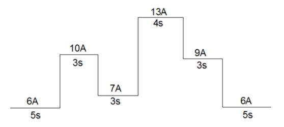
APM DC E-load could loaded according to edited waveform
